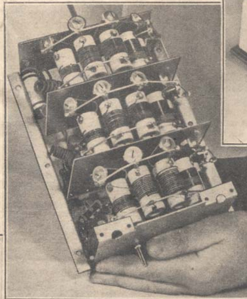
—receiver; (above) coil assembly for a five-band receiver; (left) triple gang band-spread condenser; (right) magazine soldering iron, fed from a coil of solder wire housed in the handle.
