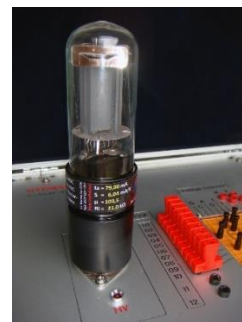
Figure 7 Accuracy check of the uTracer with a special 'bogey' calibration valve (courtesy Kurt Schmid)
