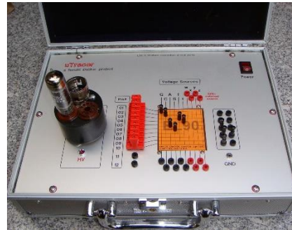
Figure 6 Kurt Schmid has designed a beautiful case for the uTracer. He used a crossbar switch to connect the uTracer to the valve and a modular socket system
