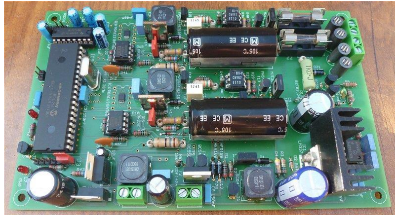
Figure 3. The complete \mu Tracer circuit fits on a 10x16 cm PCB
